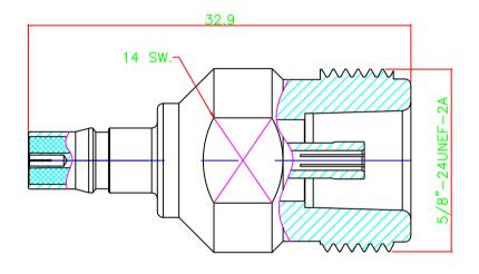
Note: Do Turn Male (Plug) Connector Nut (Shell) Only To Tighten
